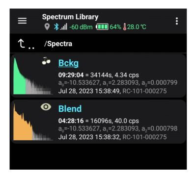
The graph of the spectrum selected for display is shown in green. For <u>8-bit spectra</u>created by a device with firmware version less than 4.00, an orange marker with the number 8 is displayed in the lower right corner.
