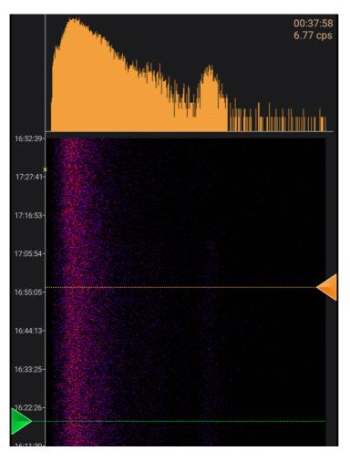
The interval is selected by dragging the triangles (markers). The scale of the spectrum (linear or logarithmic) corresponds to the scale selected for the spectrogram.
