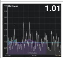
Graph of radiation hardness. It is formed from log data and operational data (gray zone), allows you to estimate the conditional radiation hardness for a specific device model. It is displayed as a dimensionless coefficient, which is calculated as (µrem/h)/(cps).
