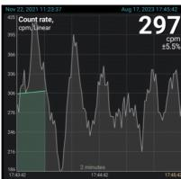
Pulse count rate graph. The start and end date/time of the data section loaded into application memory from the database is displayed in blue at the top of the graph. This portion of the data is available for display in the graphs.
