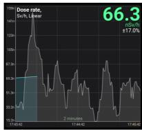
Dose rate graph. The units of measurement are selected in the device settings. When an alarm occurs, the dose rate value is displayed in the color corresponding to the alarm.
