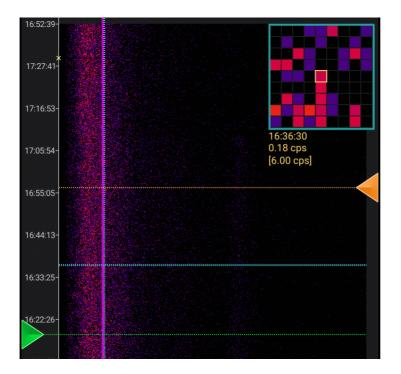
Under the magnifying glass the information about the spectrum channel that is in the center of the magnifying glass is displayed: its corresponding time or count number, count rate (number of pulses in this channel divided by spectrum accumulation time) and, in square brackets, total count rate for the spectrum (sum of pulses in all channels divided by accumulation time).
