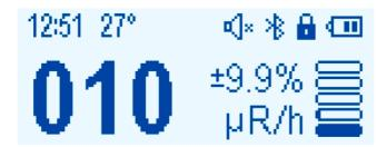
This is a screenshot of the device screen, which is updated every two seconds. When an alarm occurs, the widget can be updated more frequently. You cannot change the size of the device screen widget.
