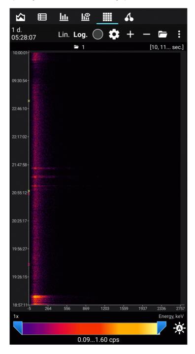
Each line on the vertical (Y scale) is a separate spectrum typed in the "Capture Interval". The size of the interval can be set in the settings. The horizontal (X scale) shows either spectrum channel numbers or photon energy calculated by analogy with the Spectrum tab. The count rate in each individual channel (Z scale, similar to the Y scale in the Spectrum and View tabs) is converted to a
